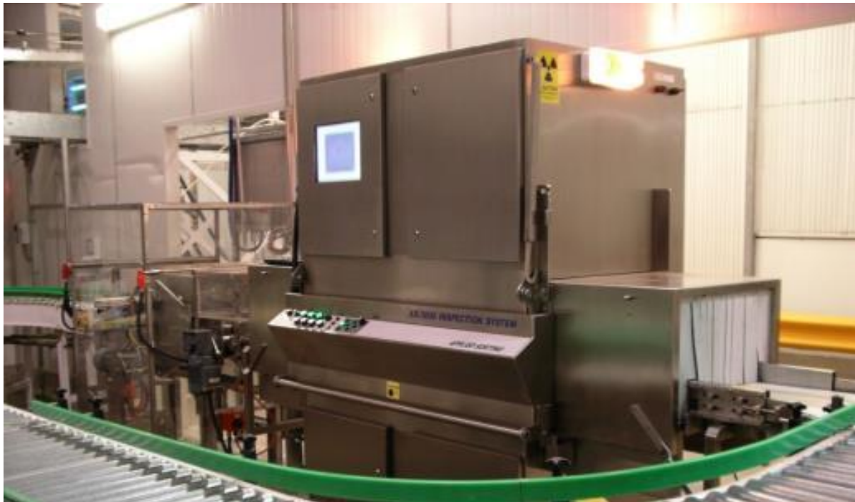
Figure 1 - XR-3000 X-ray Inspection Machine - the platform for the beef bone belt DEXA system
