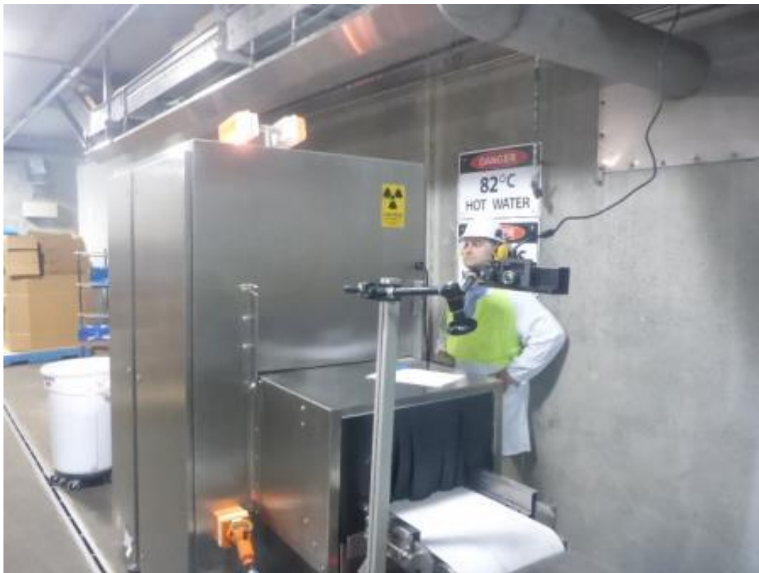
Figure 24 - Bone Belt DEXA machine installed at the customer's site
