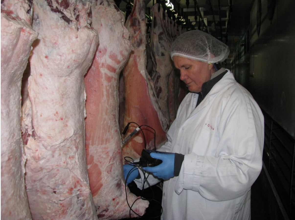
Figure 1: Measuring the pH of a lamb carcass
