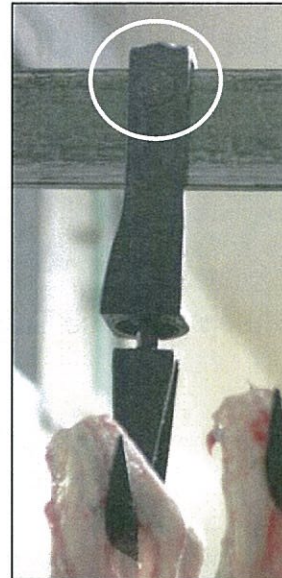
1: SCL injection moulded HF transponder on gambrel
