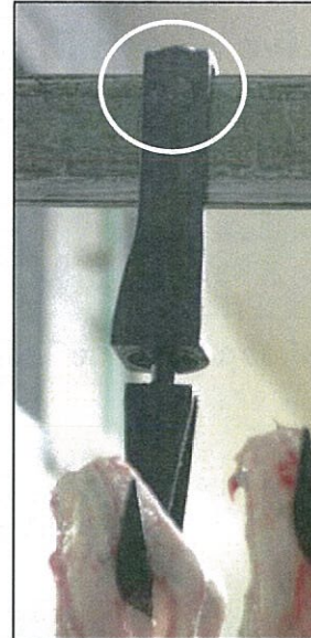
1: SCL injection moulded HF transponder on gambrel
