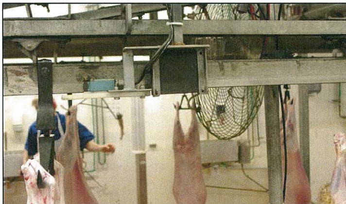
3. Kill floor Electrocom gambrel HF RFID antenna and FEIG® reader. Proximity switches for the pre/post-read blocker for the Allflex LF EID reader are also installed at this location.
