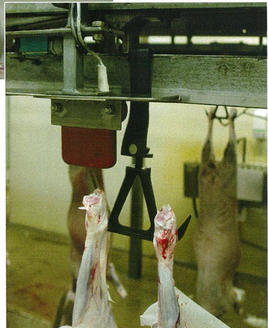
SCL Encased Sunshine Technologies HF reader on the Kill Floor
