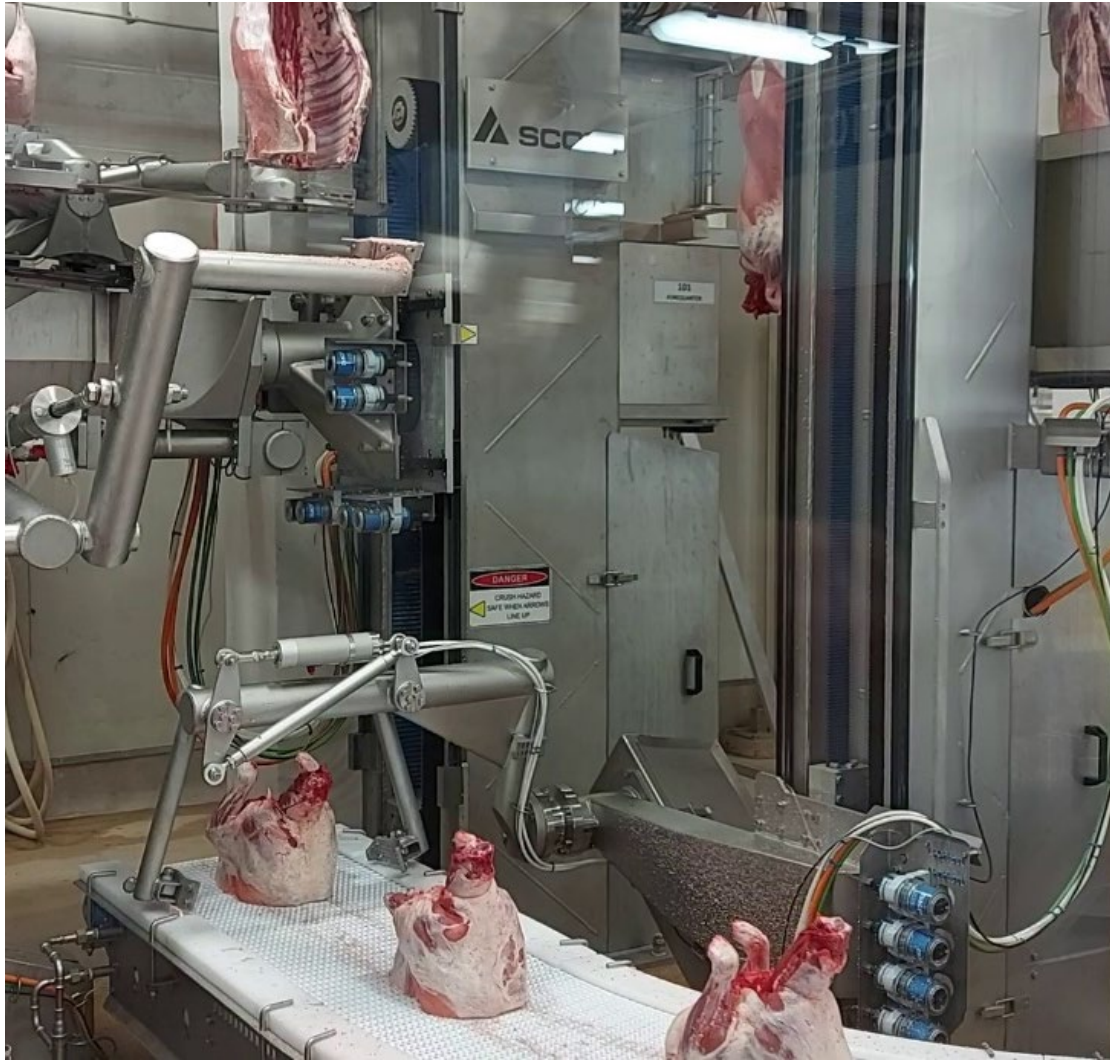
Figure 23: Forequarter integration station upgrade kit commissioning and demonstration on a production system.
