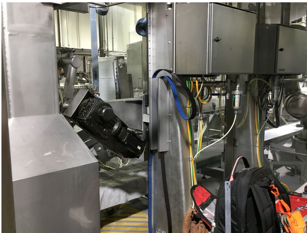
Figure 5: Main pivot has been identified as undersize for full range of Australian product.
