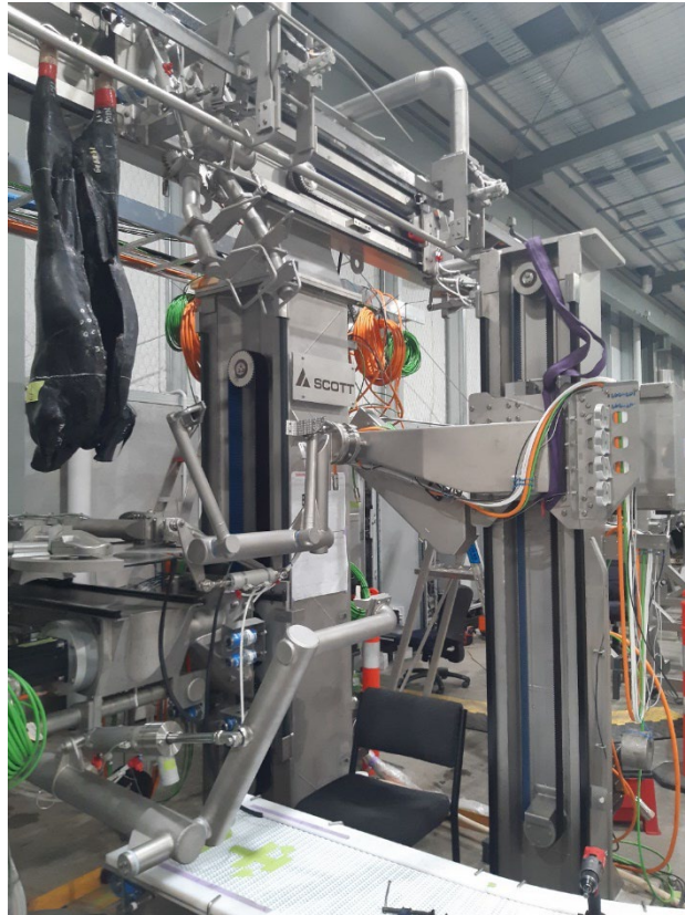
Figure 15: Upgraded forequarter integration station build implemented onto a recent system assembly.
