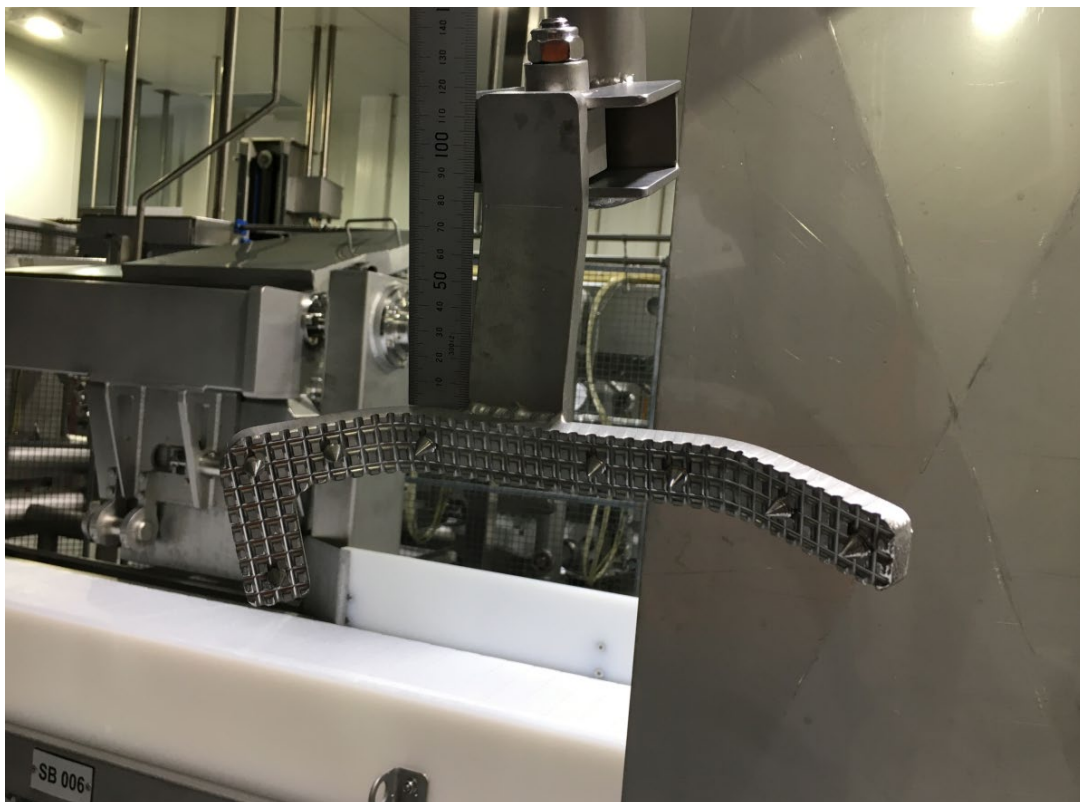
Figure 10: Example where gripper design is being assessed for effective product handling.
