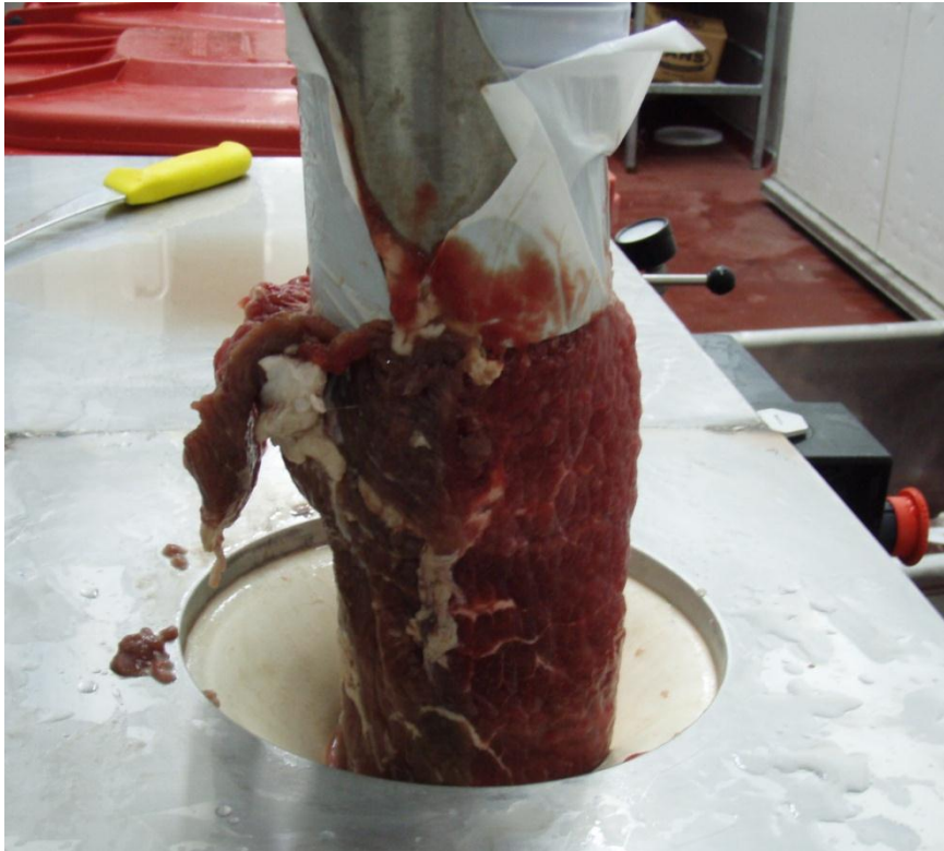
Figure 7 Costs are increased from attempting to form product into a casing size that is too small.
