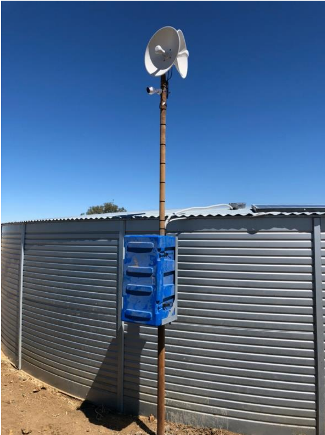
Photo 9: uSee IP tank monitor with camera and WIFI.
