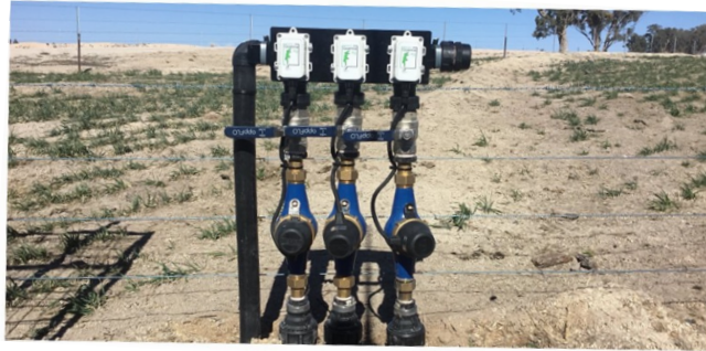
Image 7: Flow trough sensors deployed at Site 5
