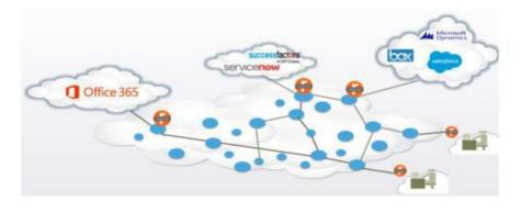
As shown above, the user's SaaS request is identified via layer-7 DPI, geo-DNS determines the tenancy location and a cloud SteelHead is automatically spun up at the closest point to the SaaS services, ensuring maximum performance irrespective of the user or the SaaS location. The Akamai SRIP (Sure-Route IP) network is also leveraged to ensure the most efficient path to the tenancy.
