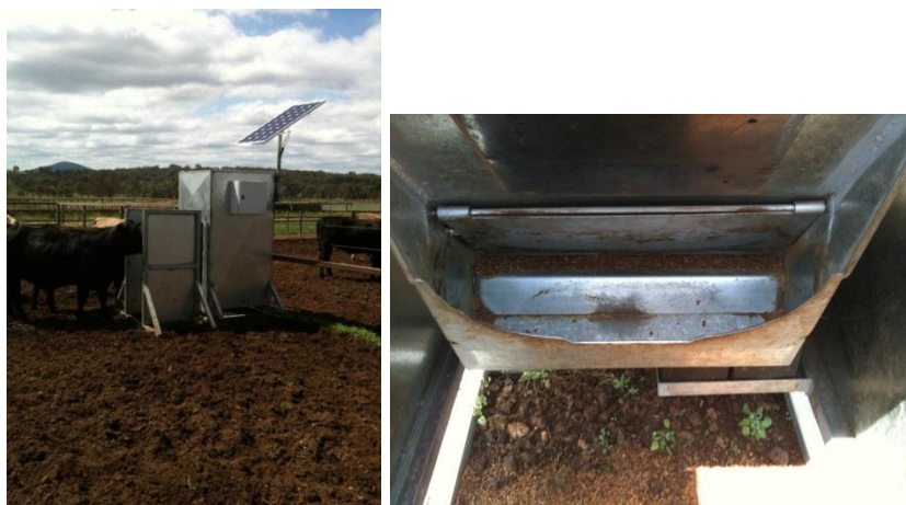
Figure 3. Second prototype bin with automatic gate with a shorter race.
