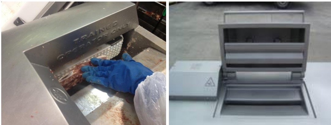
Figure 3: Rack loading mechanisms in the McLaren iFrenching system (left) and the WASSCO Frenching system (right)
