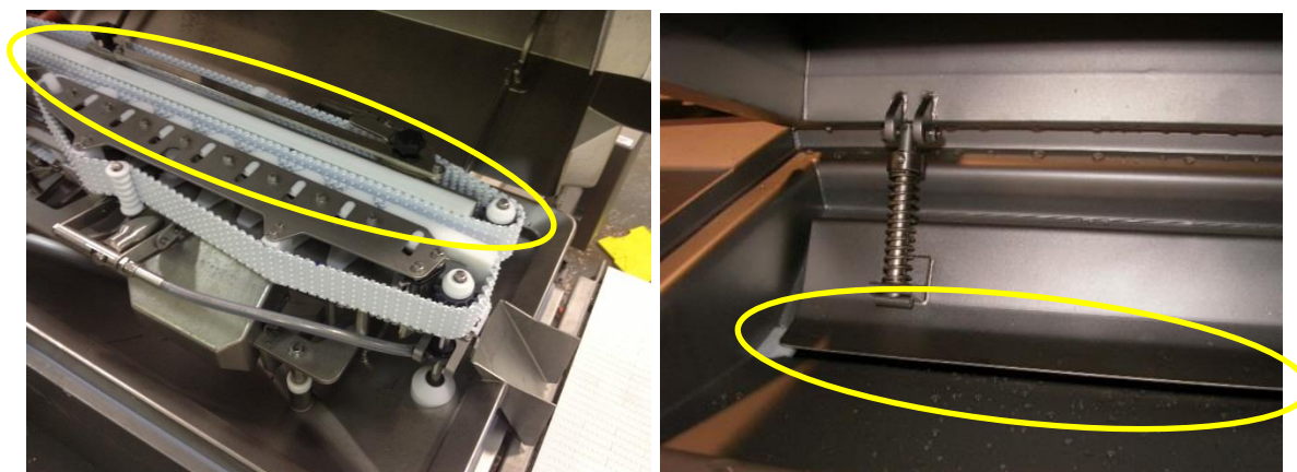
Figure 4: Rack retention mechanisms in the McLaren iFrenching system (left, Source: Green et al., 2014) and the WASSCO frenching system (right, Sources WASSCO, 2014a)
