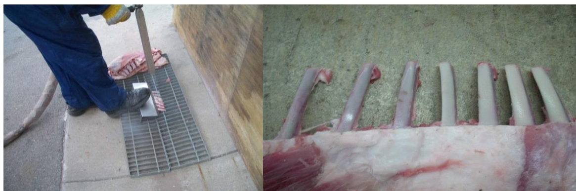
Figure 6: CO 2 Frenching trial being conducted (left) and the frenched rack as a result (right) (Source: Hart, 2010)
