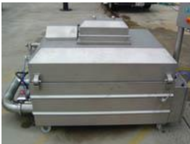
Figure 10: The WASSCO frenching system has a foot print of 1.5m 2 (Source: WASSCO, 2014b)
