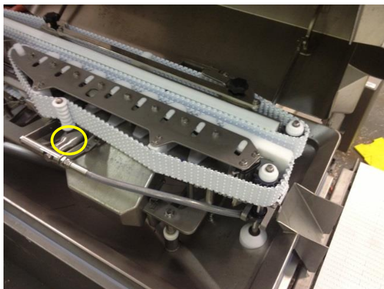
Figure 5: Water frenching jet of the McLaren iFrenching system (circled in yellow), (source: 2014)
