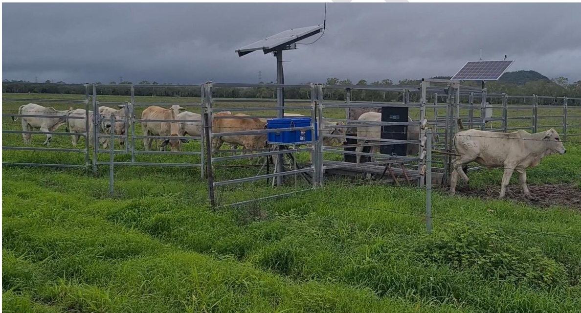
Figure 38. Heifers using the walk over weigh unit in February 2021.
