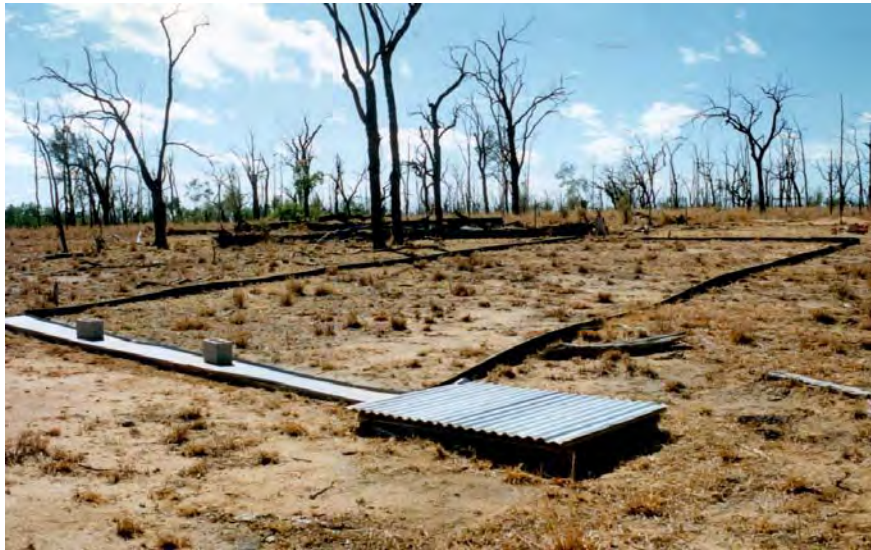
Figure 9.2 Picture of a bounded 7 x 20 m plot with Gerlach trough and runoff equipment in the foreground, from a high grazing pressure treatment paddock at the ironbark site.
