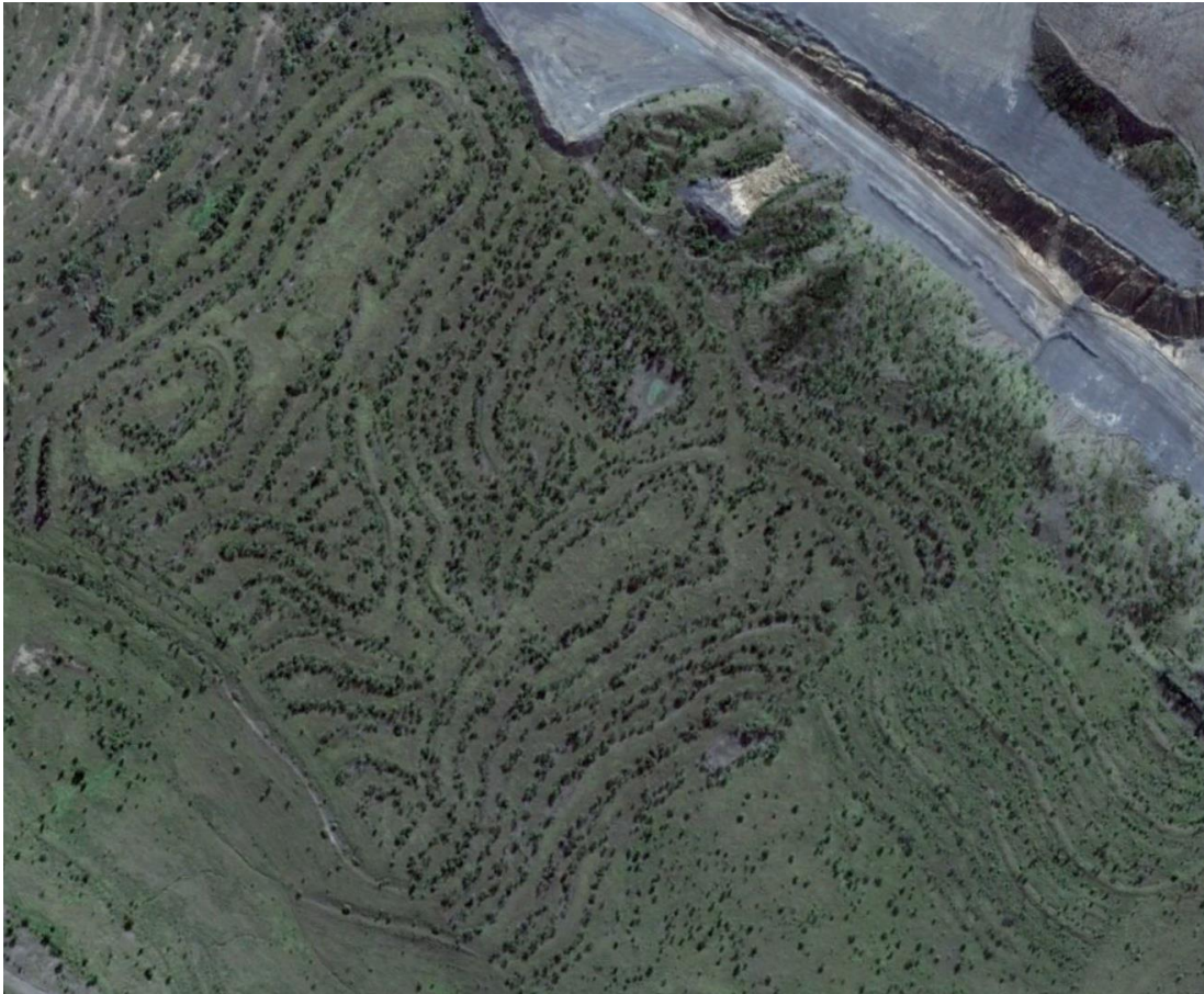
Figure 20: An example of tree-lined contour establishment at Curragh Mine (Google Earth 06/2016; -23.454539, 148.869129). Tree belts are approximate 8 metres wide and the distance between the edges of tree-lined contours ranges between 12-17 metres.
