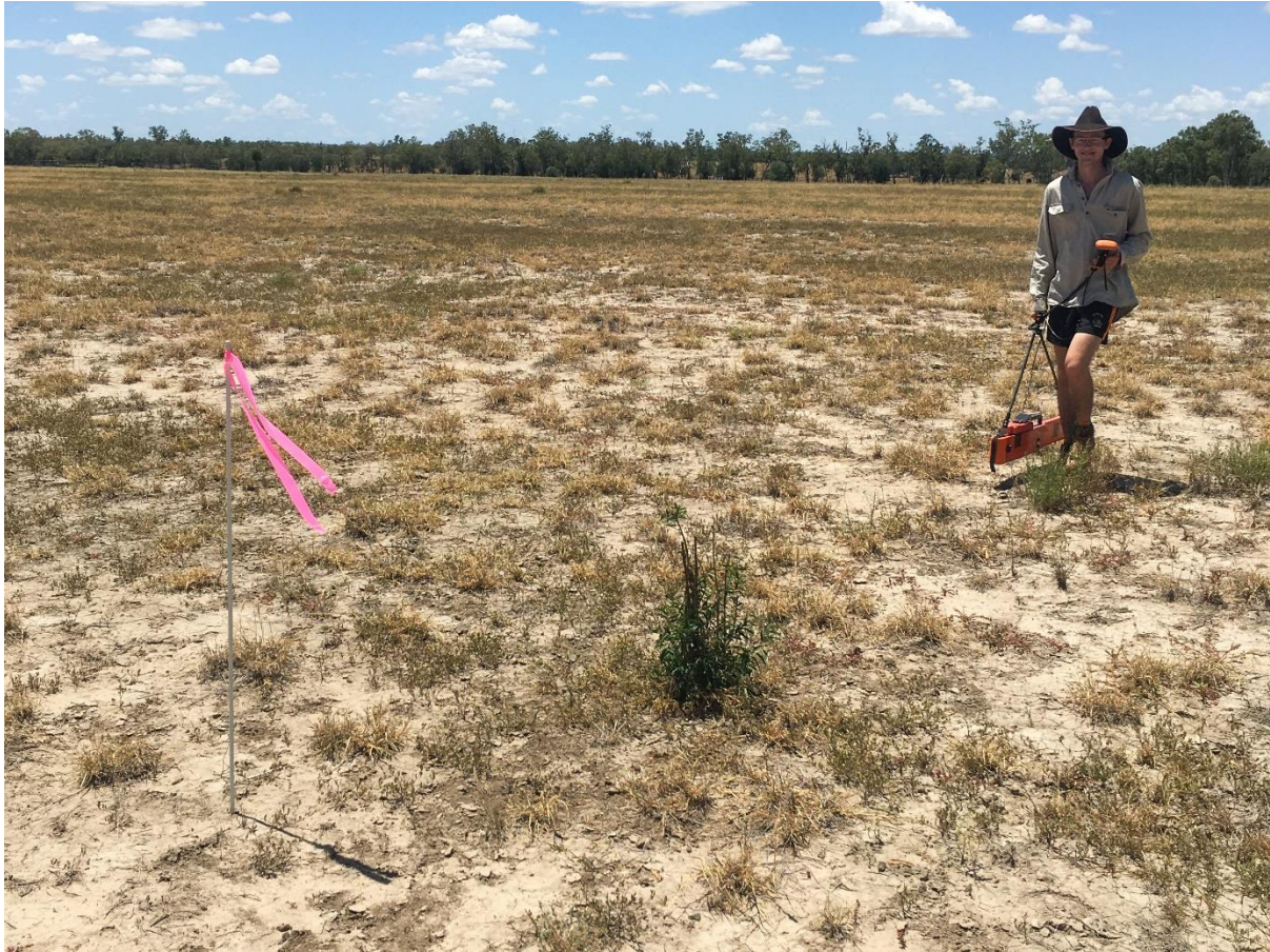
Figure 42: Measuring the sub-surface soil variation with an EM-38. Significant variation could affect trial results when they are put in place.
