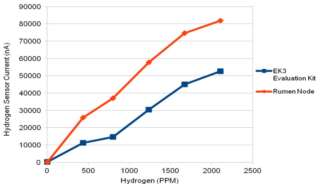
Figure 11. Gas concentration measurements using the EK-3 evaluation board and the new intra-rumen hydrogen sensor node under *in vitro* conditions.
