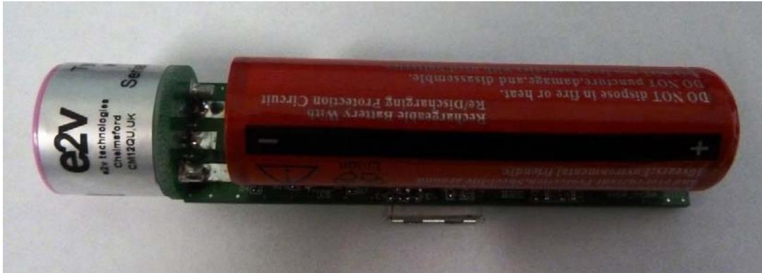
Figure 10. PACP hydra Intra-rumen hydrogen sensor node. The silver sensor is 20 mm x 20mm in dimension
