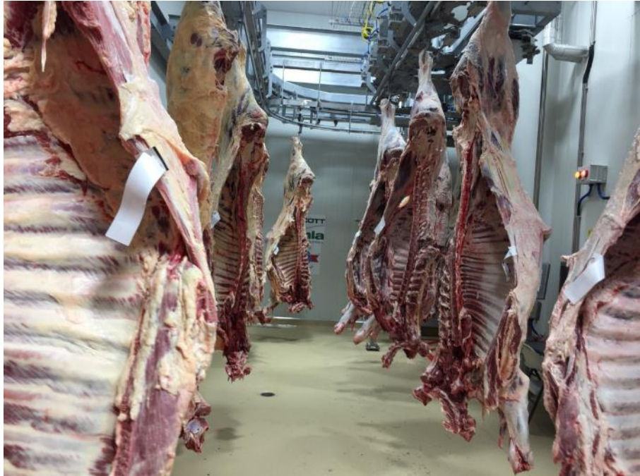
Fig. 3: Standard overhead chain conveyance of beef sides.
