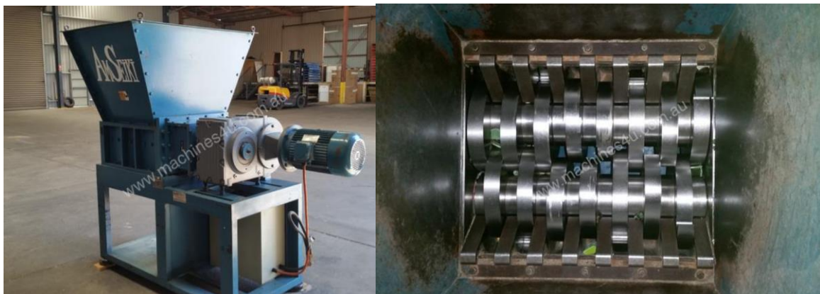
Figure 4: Example of a shredder for creating 20 mm particles from solid waste.
