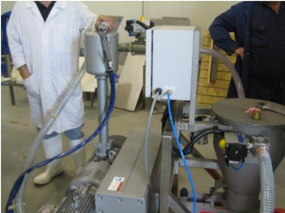
Photo 1: Modified ovine spinal cord removal system.
