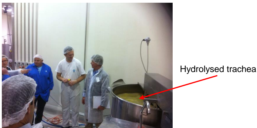
Figure 3. Jacketed mixing vessel used for proteolytic hydrolysis of minced trachea.
