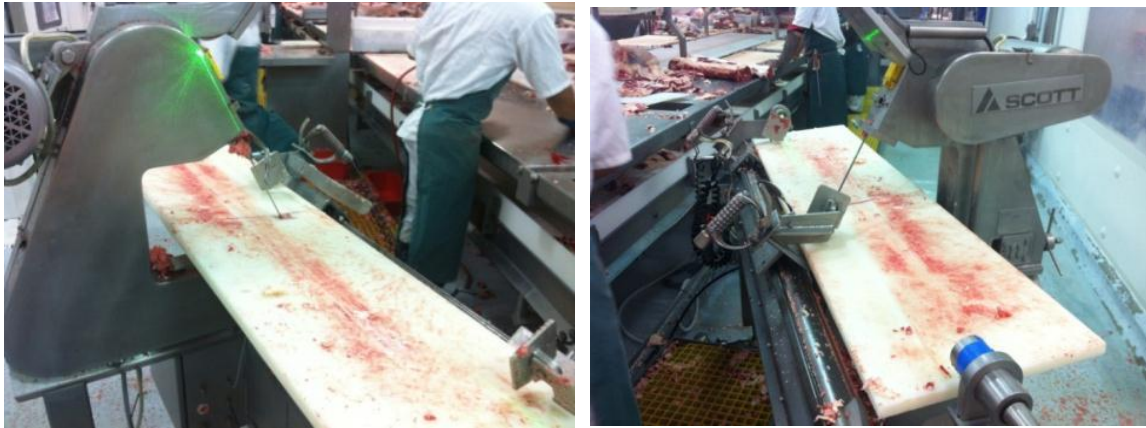
Figure 32: Integration of system into processing line will be required so operator does not have to pivot 180 degrees
