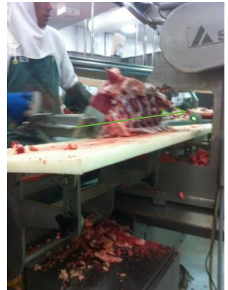
Figure 31: straight cutting line is easier for operator but could impact on yield slightly compared with generic saw although this was not evident in the data collected
