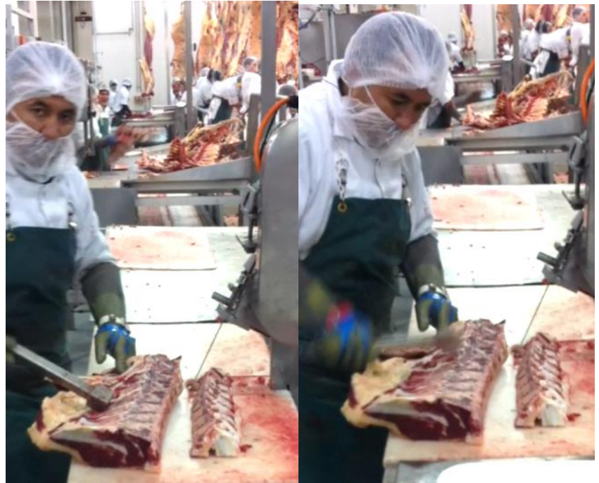
Figure 29: Steel mallet used to force the separation of ribs from vertebra where cut leaves ribs joined
