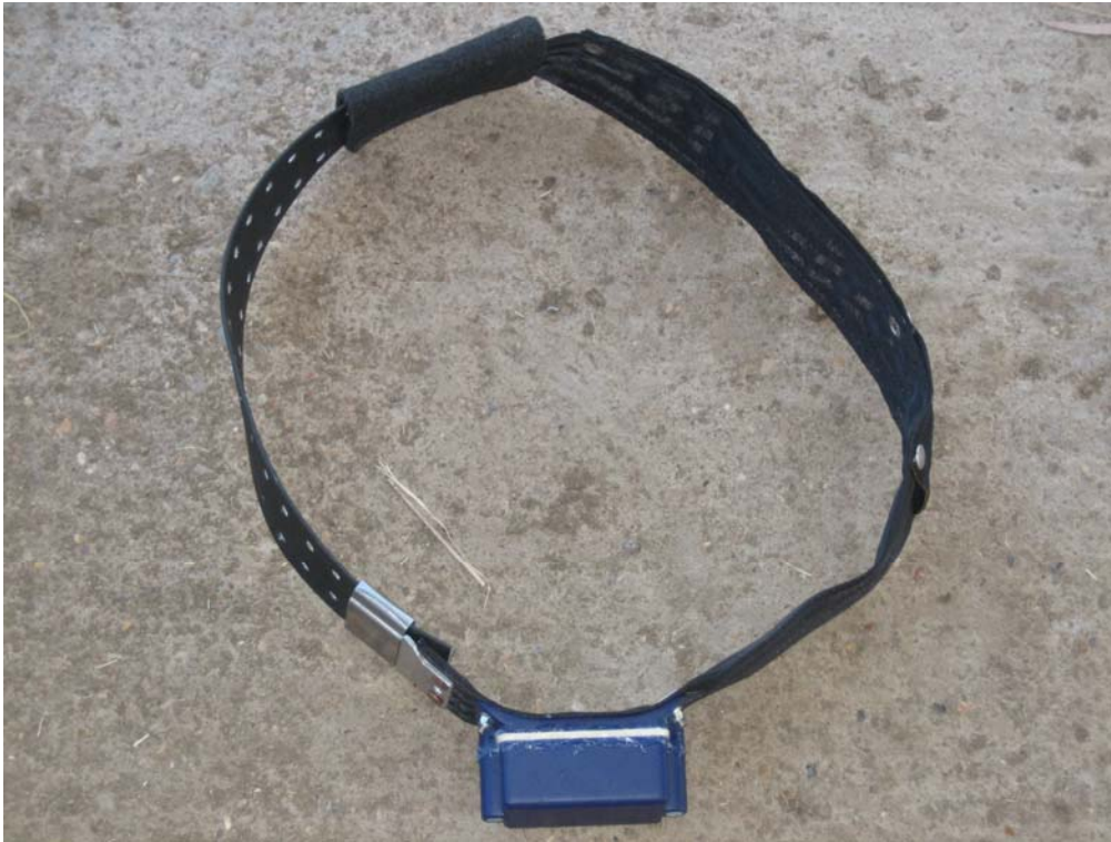
Figure 4.10 GPS collars have been re-designed to facilitate better placement of the GPS antennae and easier fitting to animals
