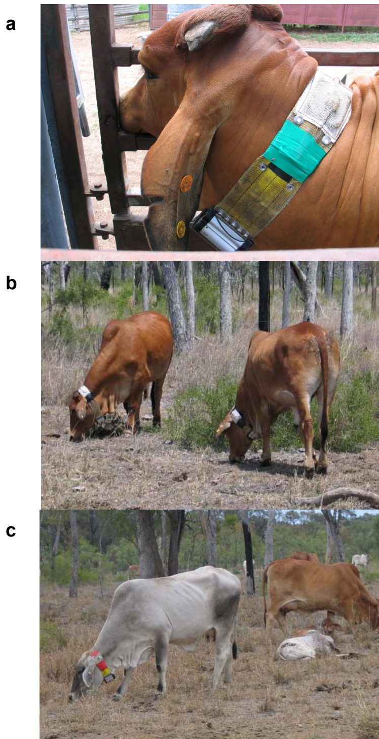
Figure 3.2. GPS units fitted to grazing cattle. a) Detail of unit on animal, b) units on Brahman cross steers, Wambiana and c) on Brahman cows in a commercial sized paddock
