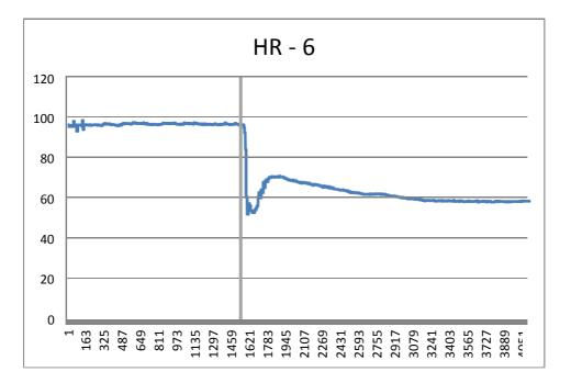
**Figure 5**. Typical ECG pattern after microwave application, recorded from Animal six receiving 20 kW for 10 sec. The time of microwave application is indicated by the grey shading. Time is counted from the start of the microwave application.
