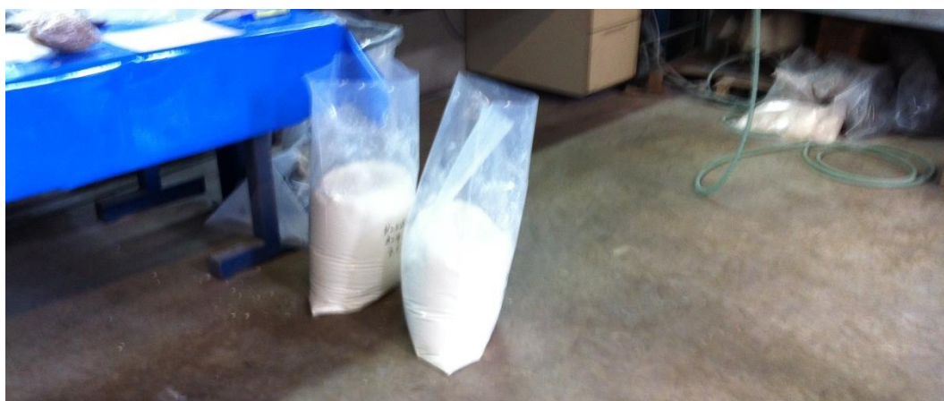
Figure 6. Extracted bone powder following a first pass with the standard rotor (left) and a second pass with a fine rotor (right)
