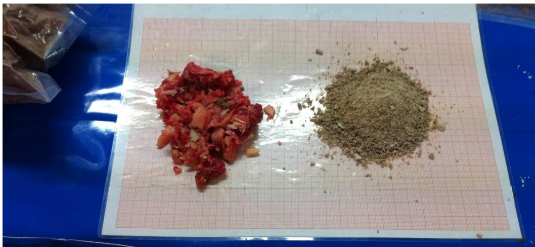
Figure 8. 50:50 crushed bone and 90 CL trim before and after 1 pass of the mill
