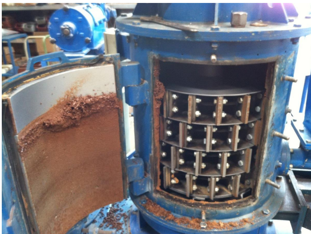
Figure 3. Product build up inside the Turbo-rotor mill processing 90 CL trim
