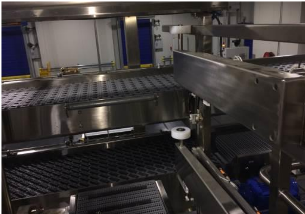
Fig. 5 Divert gates used to diverted cartons off the main ring. This image shows the infeed conveyor set to receive cartons off the lower (chilled) ring conveyor.
