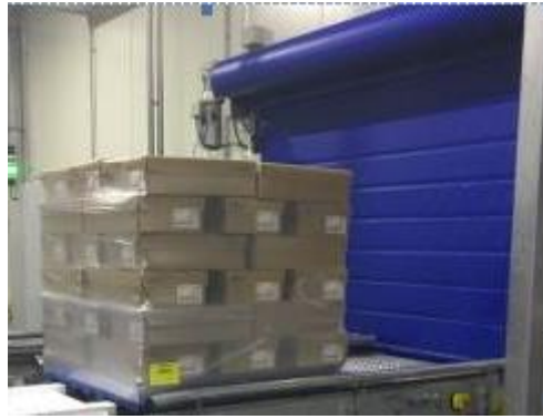
Fig. 10 Wrapped pallet complete with pallet label deposited at entrance to freezer
