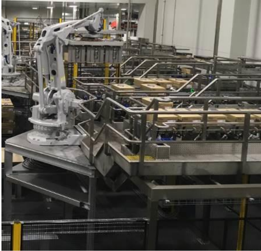
Fig. 3 Robot and gripper with cartons queued on infeed lanes ready for palletising
