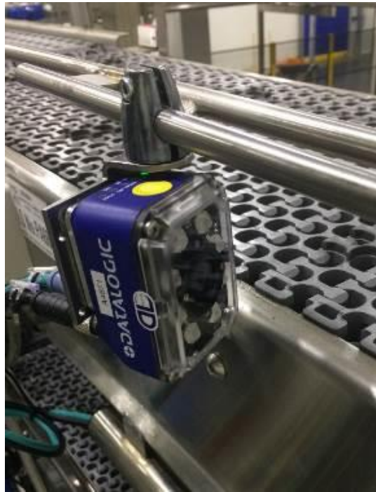
Fig. 4 Barcode scanning camera on the main ring, used to determine which infeed lane each carton should be diverted down.
