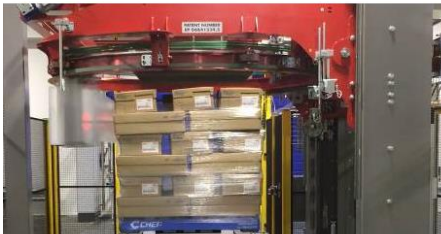
Fig. 9 Completed pallet being wrapped
