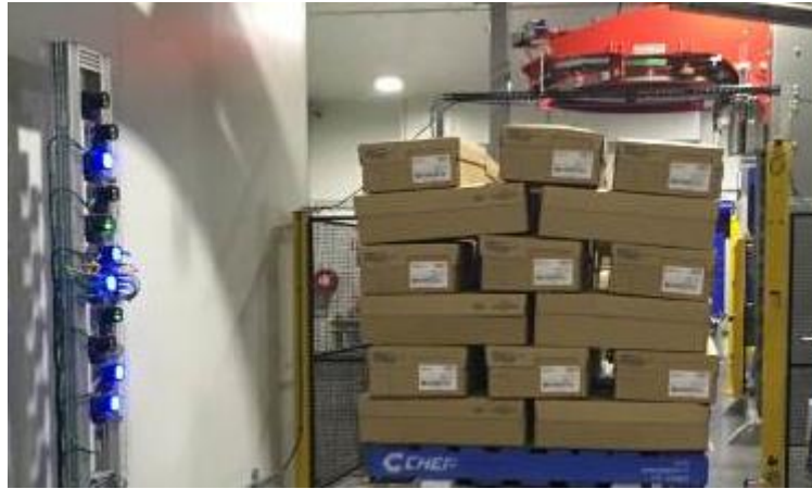
Fig. 8 Completed pallet ready for scanning by the Pallet Barcode Scanning System
