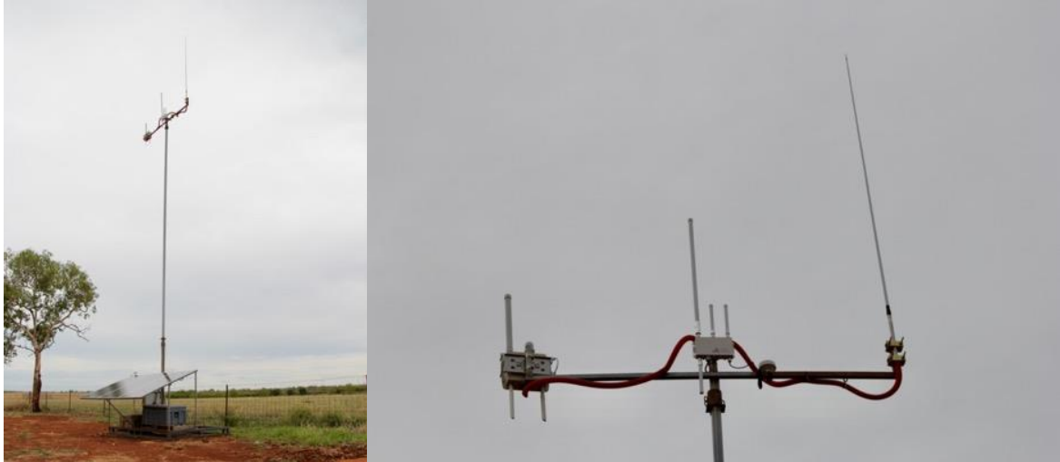
Figure 4. Photo of transportable tower with 8m mast manufactured by Katherine Research Station staff.
