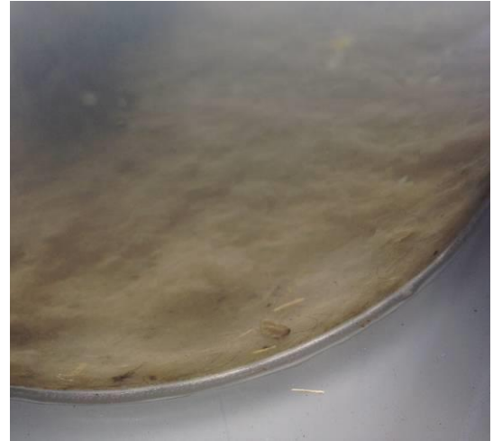
The same paunch material post sonication has largely settled to the bottom of the vessel 1 hour after processing.
