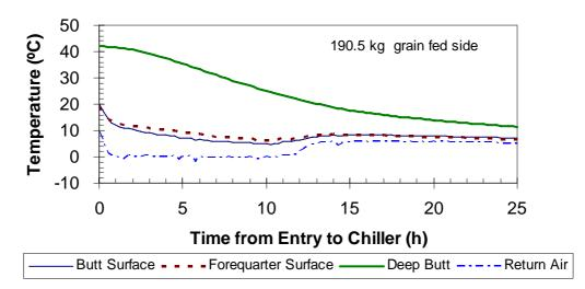
Figure 1: Typical current chilling cycle for beef sides
