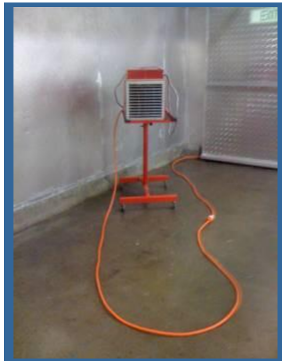
FIGURE 1. Hotbox-Axial Blower Heater HB90415—415V 9.0kW in small chiller B - wet floor pre heating.
