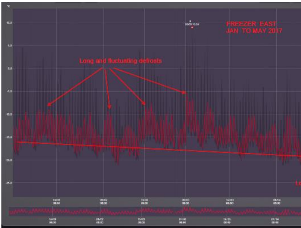
Figure 3 - Freezer East Temperatures - showing long and fluctuating defrosts.
