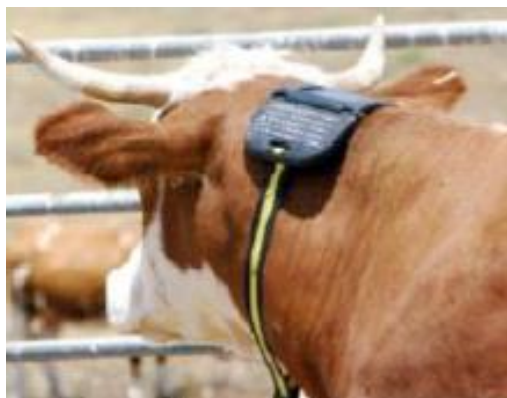
Figure 5 The prototype Cattle Sense® collar, complete with solar panel
