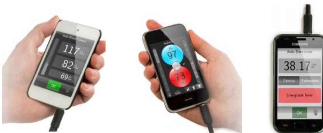
Figure 14 LionsGate Technologies Vital Signs DSP™ (L-r, blood pressure, oximeter, thermometer)
