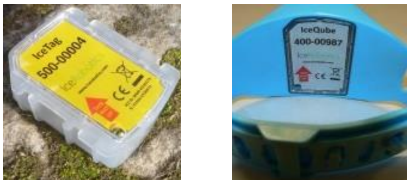
Figure 6 The IceTag (left) and IceCube (right) sensors
