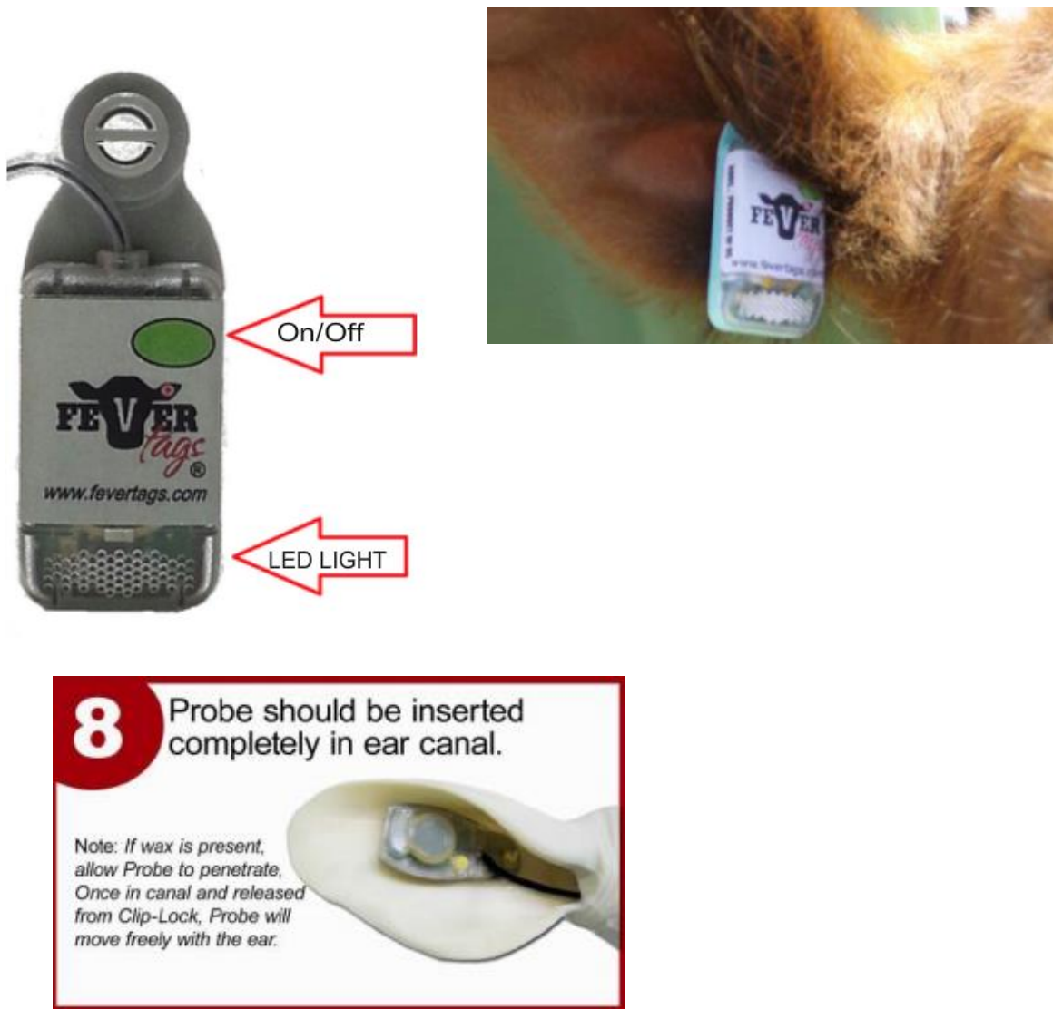
Figure 10 The FeverTags® temperature recording system
