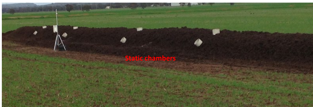
Figure 8 Static chamber measurement of fluxes from a compost row at the southern feedlot site
