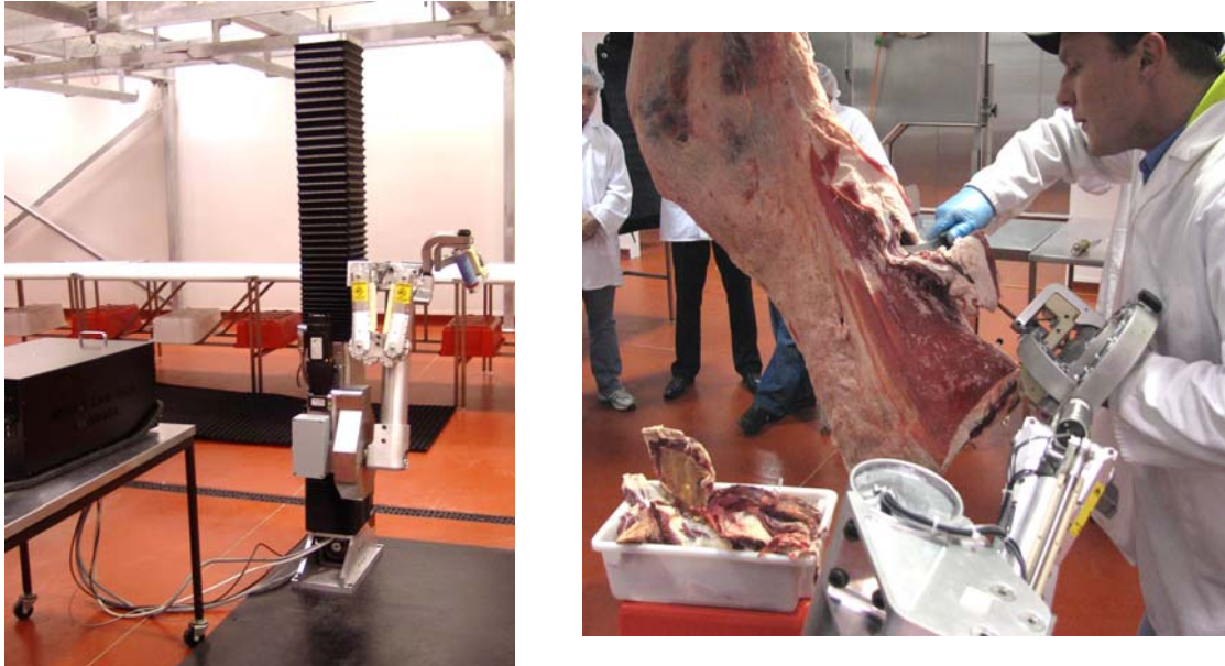
Figure 1 – (left) Picture of the HookAssist as installed at NMIT during the August 2008 Workshop. (right) Boner demonstrating use of the device.
