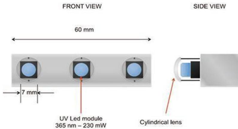
Figure13: UV-A Fluorescent Lamp Assembly for Hyper-Spectral Imaging
