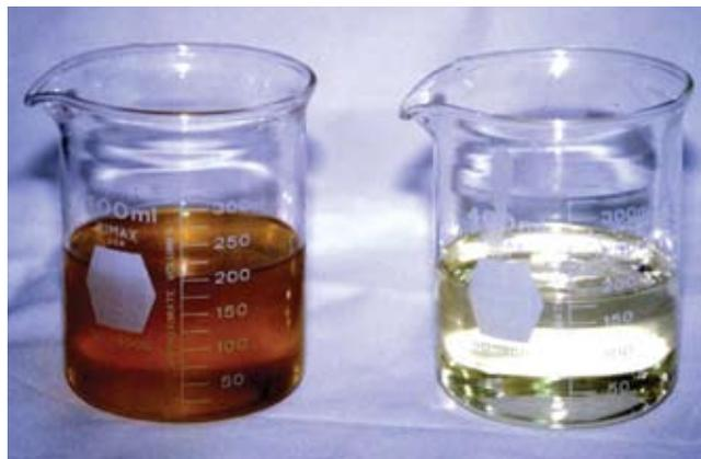
Figure 3.6: Raw and unbleached versions of a tallow sample
