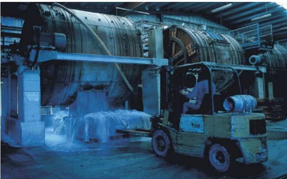
Figure 2.1: Dropping wet blue from a tanning drum
