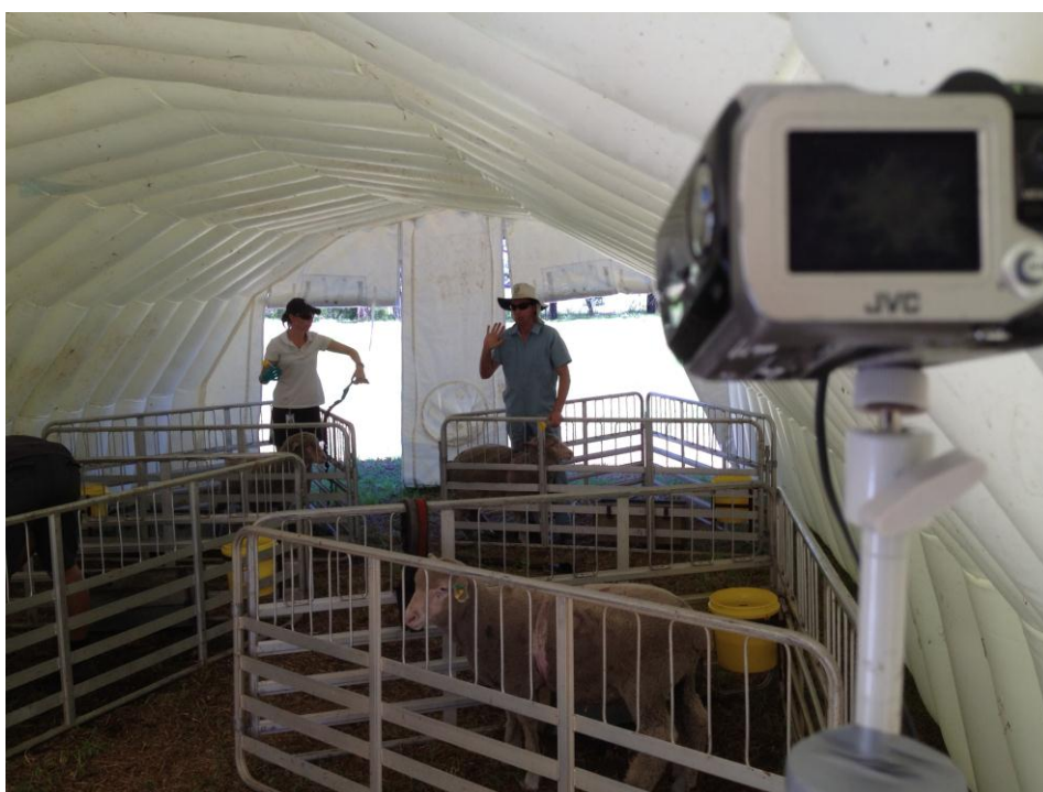
Measuring methane emissions from sheep using a polyethylene tunnel
