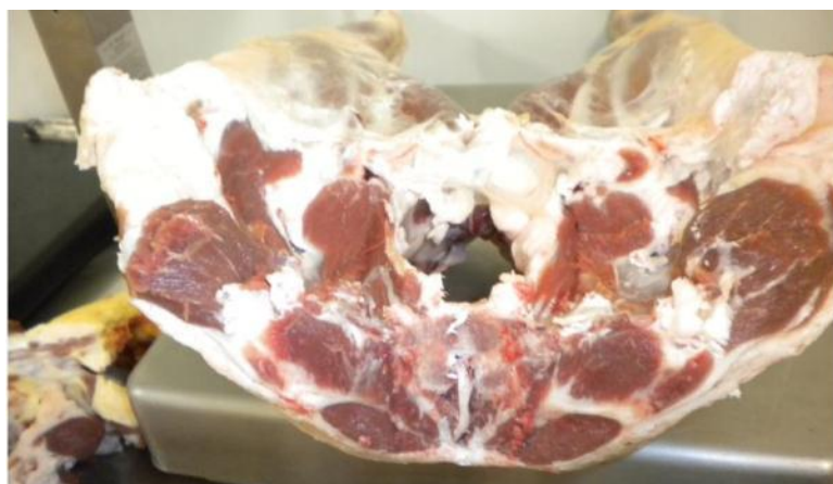
Figure 36: Lamb hindquarter cut with the LEAP III x-ray primal cutting system, note cut meat surface and lack of bone dust present.
