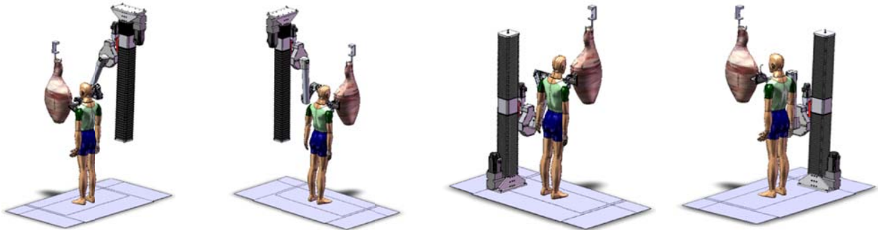
Figure 4 - Illustrations of the four different possible configurations that will be possible with the device. From left-to-right the configurations are: floor-right handed, floor-left handed, ceiling 1 -right handed, ceiling-left handed.
