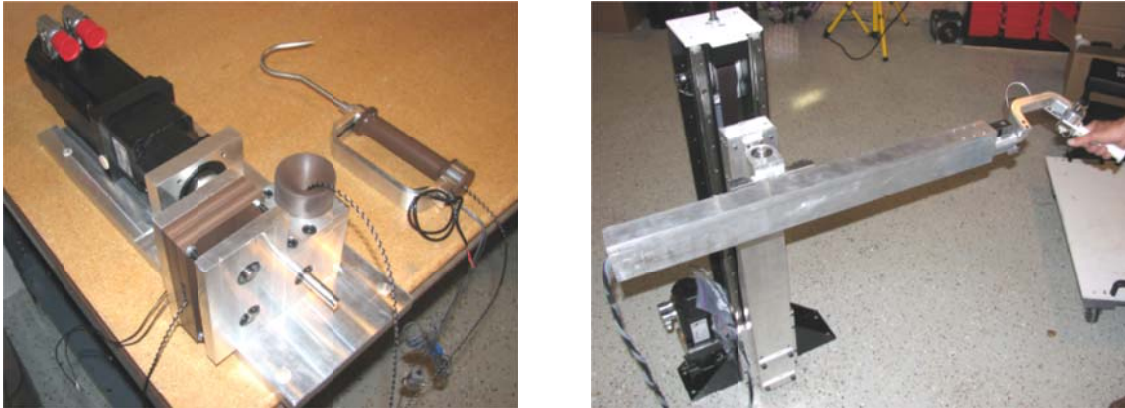
Figure 1 – (left) Picture of cable based HookAssist prototype. (right) Picture of the 'rigid arm' based HookAssist prototype.
