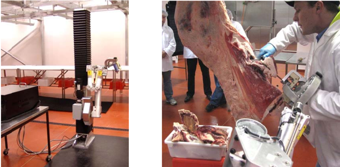
Figure 3 – (left) Picture of the HookAssist as installed at NMIT during the August 2008 Workshop. (right) Boner demonstrating use of the device.
