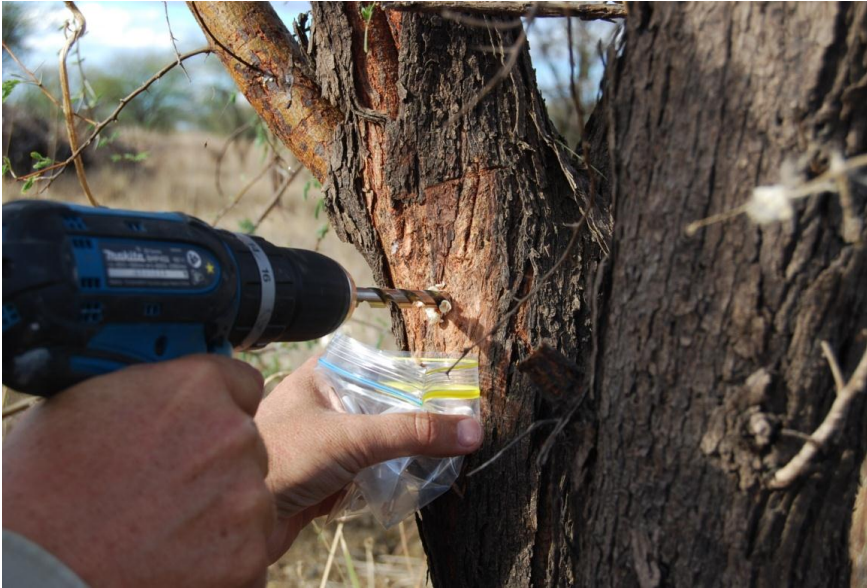
Use of cordless drill to remove samples of internal wood from a prickly acacia tree trunk – Alick Creek site
