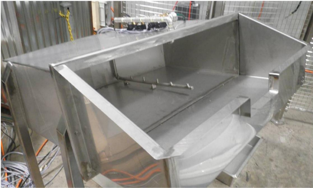
Fig. 10 Blade wash tank
