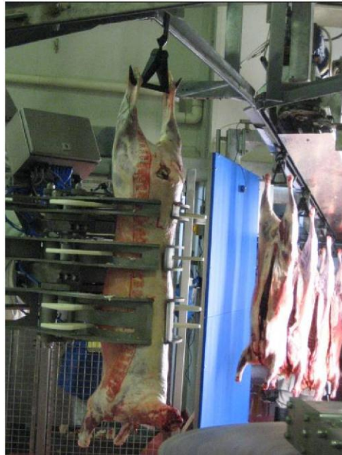
Fig. 12 Inclined carcass infeed conveyor
