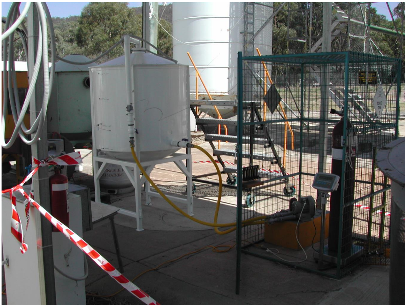
Figure 1. Sealed bin and recirculation system for treatment of one tonne of maize with EDN
