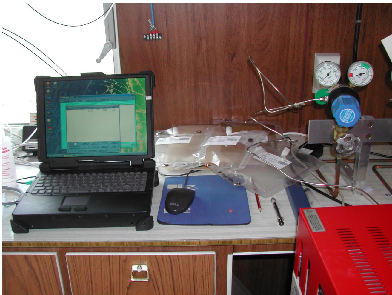
Figure 2, GC data system and Tedlar sampling bags with gastight syringe for injecting samples onto the GC.
