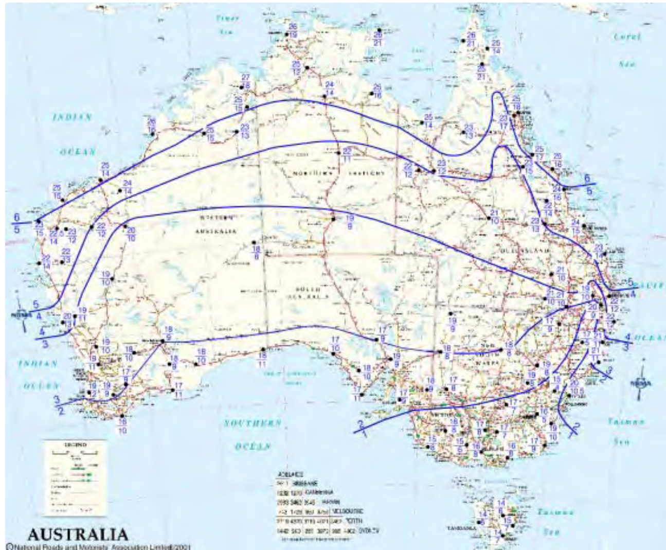
Figure 2.2 Australian Acclimatisation Zone Map with Average January (top number) and July (bottom number) Wet Bulb Temperatures at Various Sites
