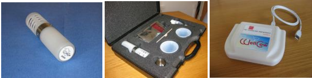
Figure 10. Well Cow bolus, calibration materials and the data reader (Source: http://wellcow.co.uk )
