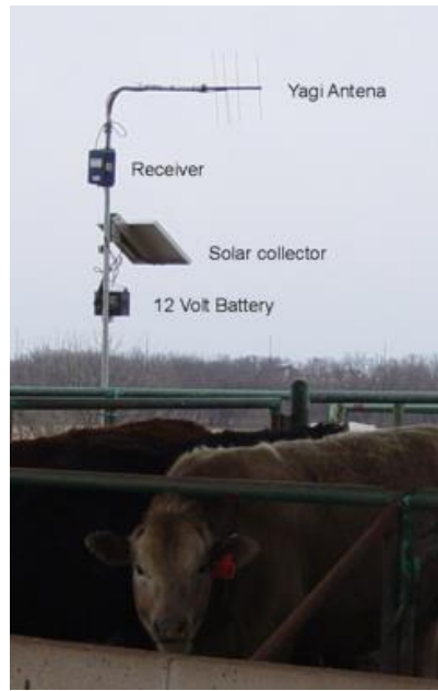
Figure 17. SmartStock™ solar receiver (Source: www.smartstock.usa.com )
