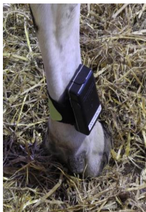
Figure 32. RumiWatch pedometer fastened on a cow's leg.
