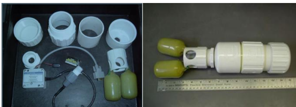
Figure 13. Illustration of the LRCpH measurement system in unassembled (left) and assembled (right) forms (Source: www.dascor.com )
