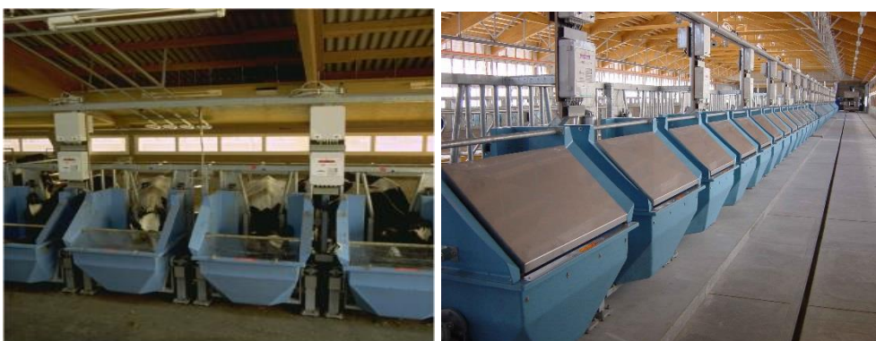
Figure 39. Roughage Intake Control (Source: www.insentec.eu )
