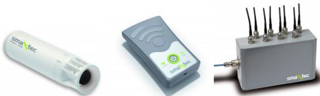
Figure 9. Smaxtec® rumen bolus, mobile reader and base station (Source: www.smaxtec.com )
