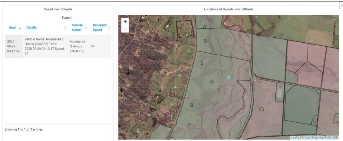
FIG 17: Vehicle Overspeed concept, where the Motorbike was limited to speed threshold of 50 Km/hr for safety. There was an alert and location noted of when the bike broke the speed threshold.
