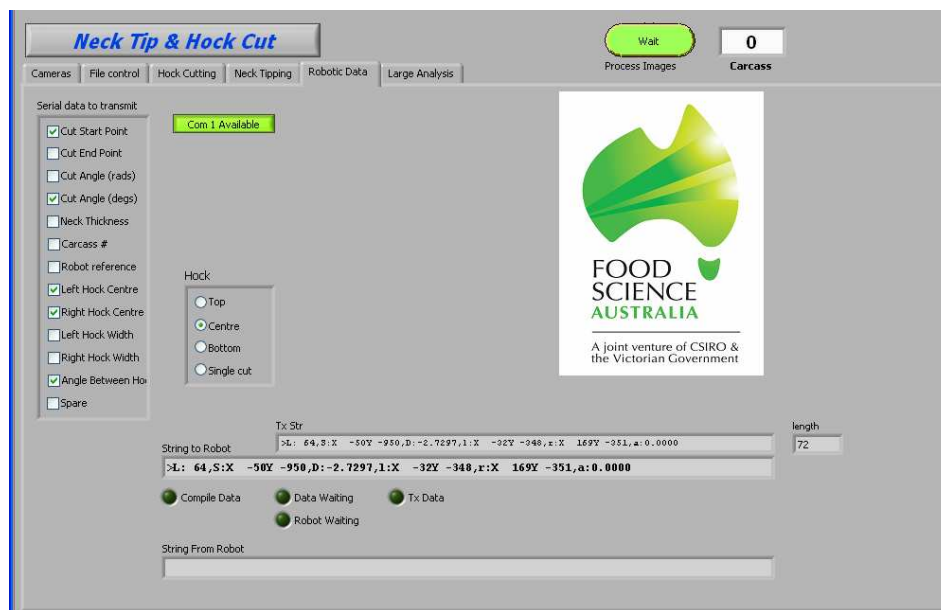
Figure 48: Analysis of the neck is integrated to the hock analysis and all the data becomes available for transmission to the cutting tool
