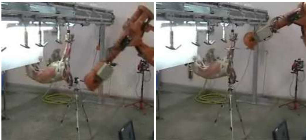
Figure 53: Neck tip and hock cut during demonstration
