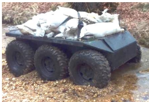
Figure 2 – Picture of MadDog, a battery only wheeled initial prototype
