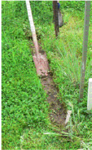
Figure 2a. Half to 1 cm of soil was removed with a sharpened spade.
