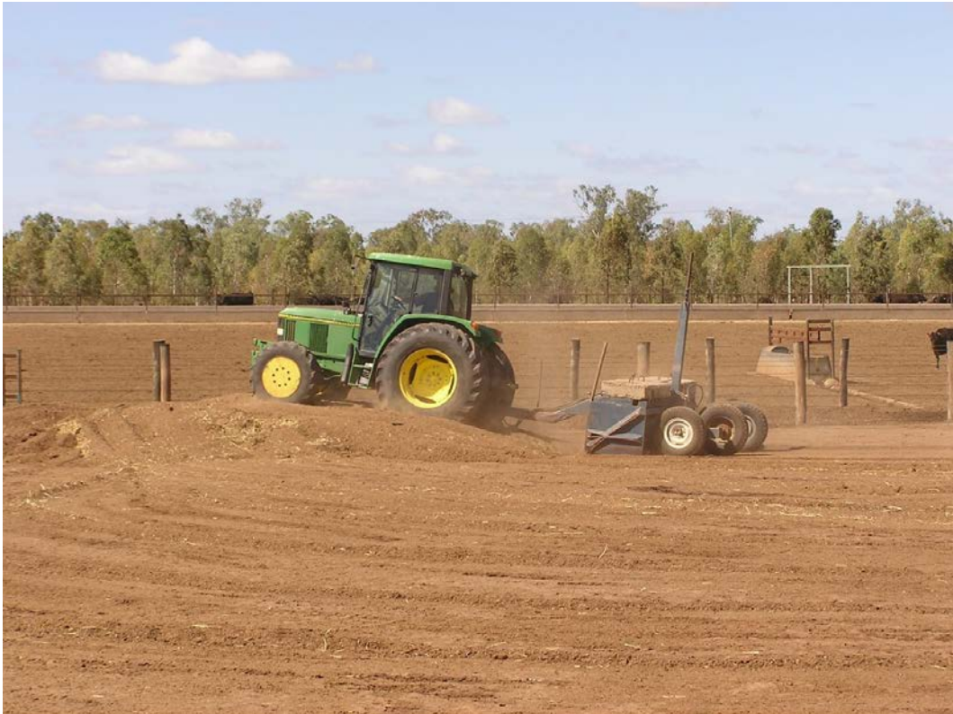
Photograph 9 – Pen cleaning under dry conditions – mounding dusty material
