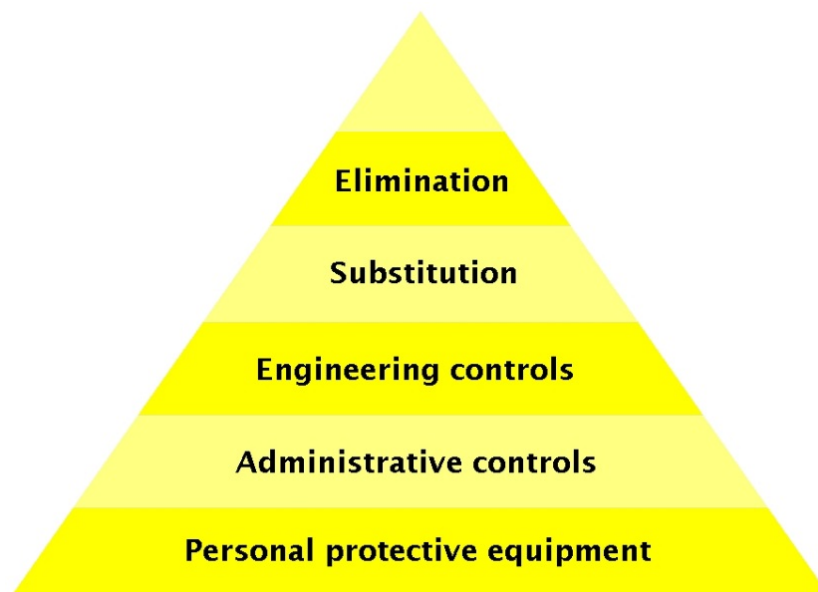
Fig. 1 – Hierarchy of dust hazard control
