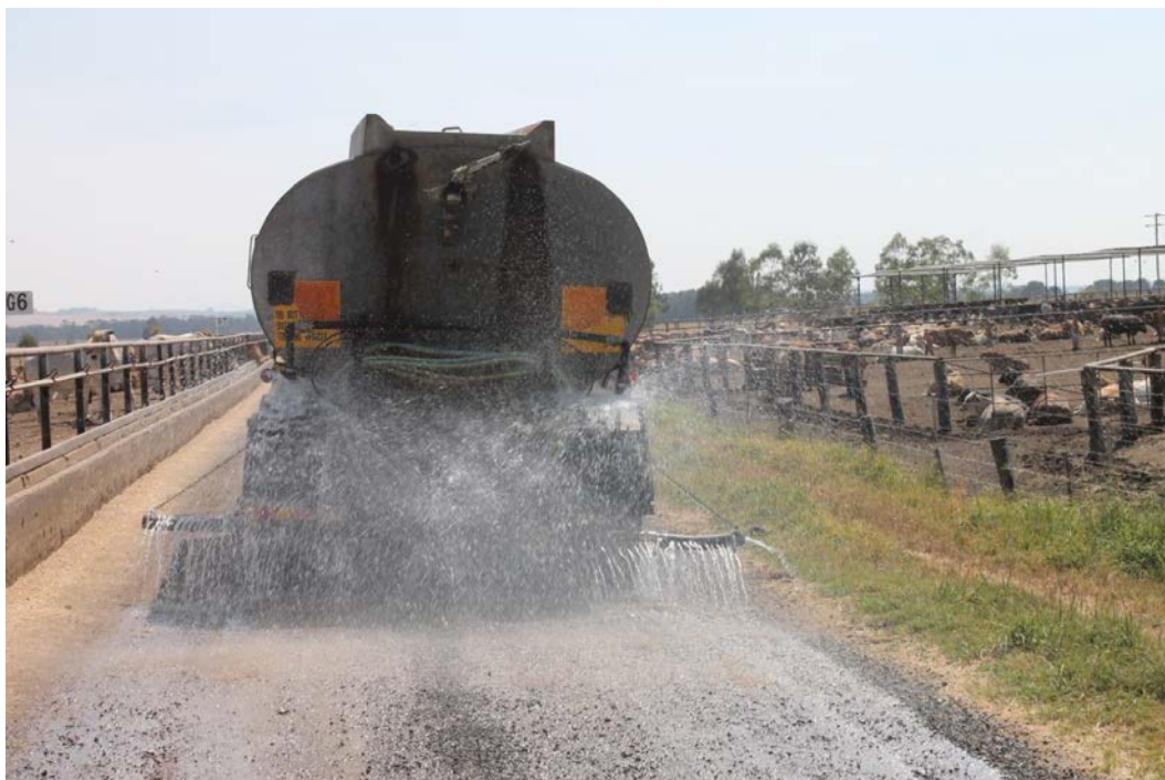
Photograph 19 – Water truck operating on gravel feed road
