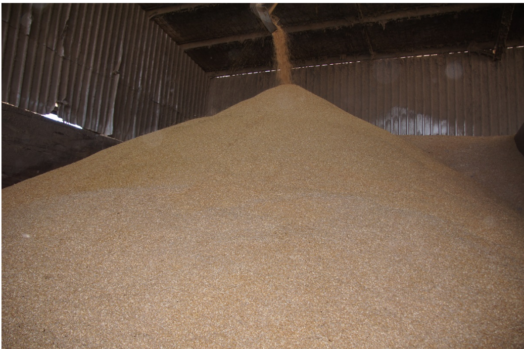
Photograph 23 – No dust from conveying rolled wet grain
