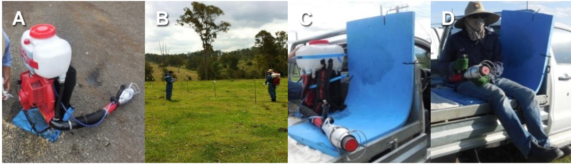
Figure 6: Field trial ULV spray application method. (A) Mistblower fitted with ULV sprayer head, (B) sprayer calibration at Pinjarra Hills, (C) sprayer mounted to utility vehicle and (D) sprayer manually operated from vehicle.
