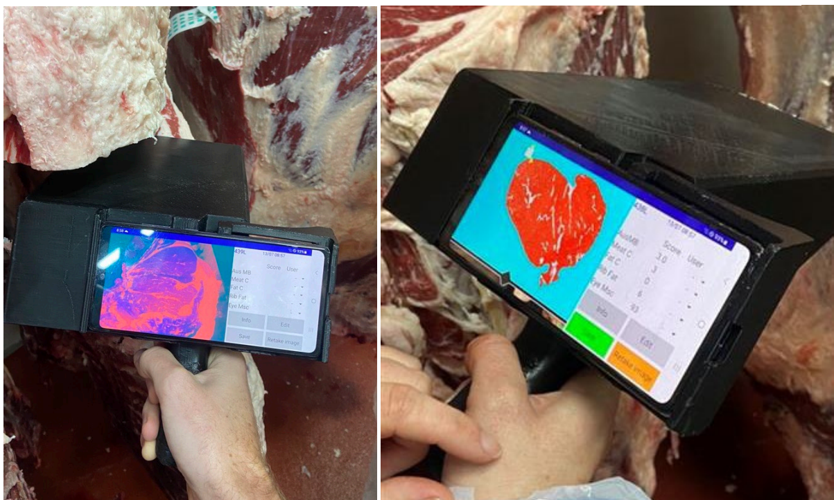
Figure 2: Masterbeef device analysing rib eye image and outputting analysis data
