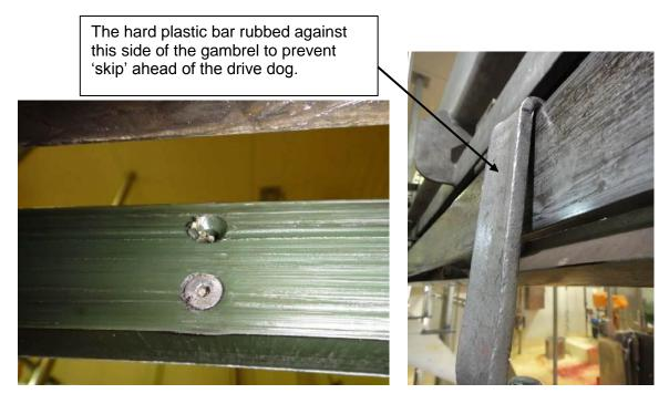
Fig. 20 Initial gambrel Stabilization used at JBS Brooklyn
