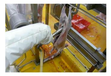
Fig.18 Carcass support bar at Peel Valley to prevent excessive movement of the carcass during fat removal
